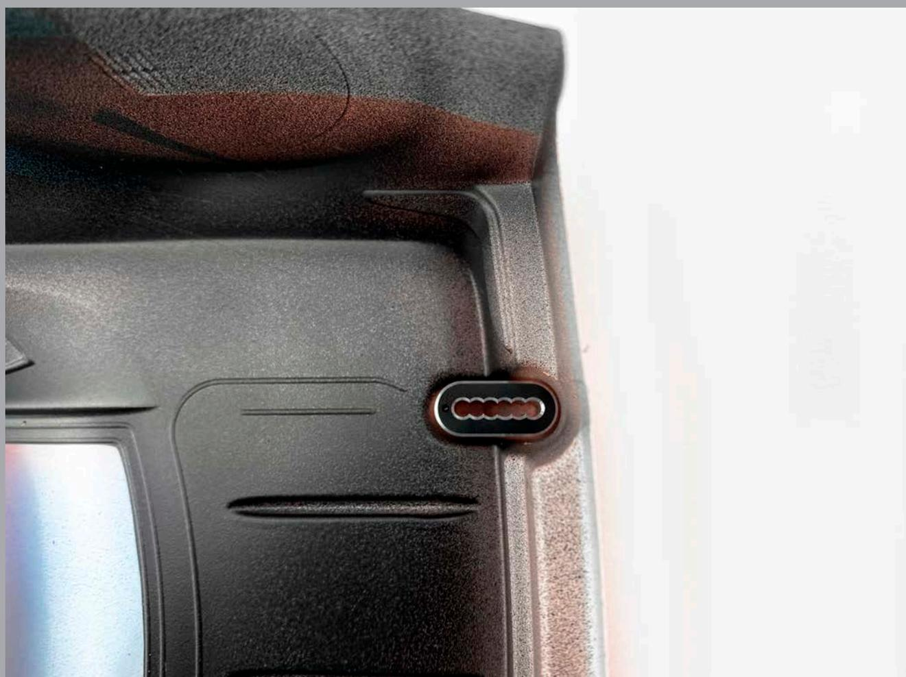
**STEP 3:** Choose your initial position to drill the hole into the Bodyshell. The hole pattern of the drill jig and the carbon plate is identically. Below we show a Precision Carbon Wing Mount plate to visualize the direction and the different positions. The gap between each hole is 2,50mm. As initial we recommend to mount the wing in the neutral position and adjust later on according the given track conditions.
