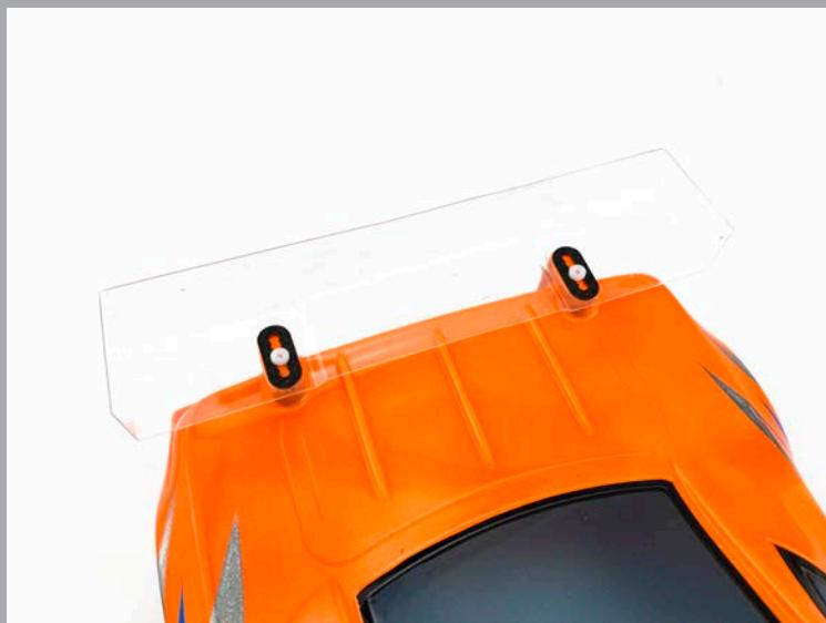
Place another Precision Carbon Wing Mount Plate inside of the Bodyshell. This extend the rigidity of the mount and keep the screw in the correct position, which is even more important if you drilled additional holes.
