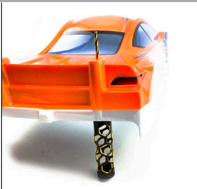
**STEP 5:** The drill jig can / should also be used to drill the holes into the wing. This will ensure a precise fitment and the best performance.
