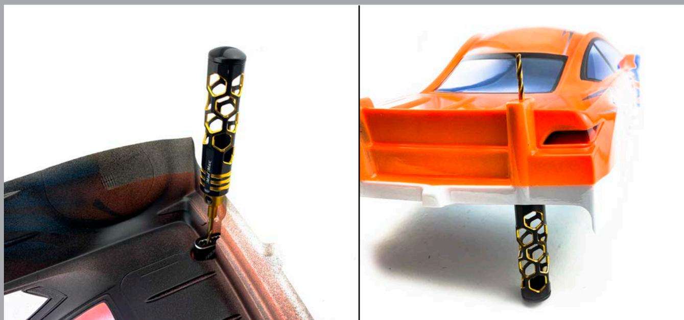
**STEP 5:** The drill jig can / should also be used to drill the holes into the wing. This will ensure a precise fitment and the best performance. We recommend to use mostly the 3rd hole from the front as shown below.
