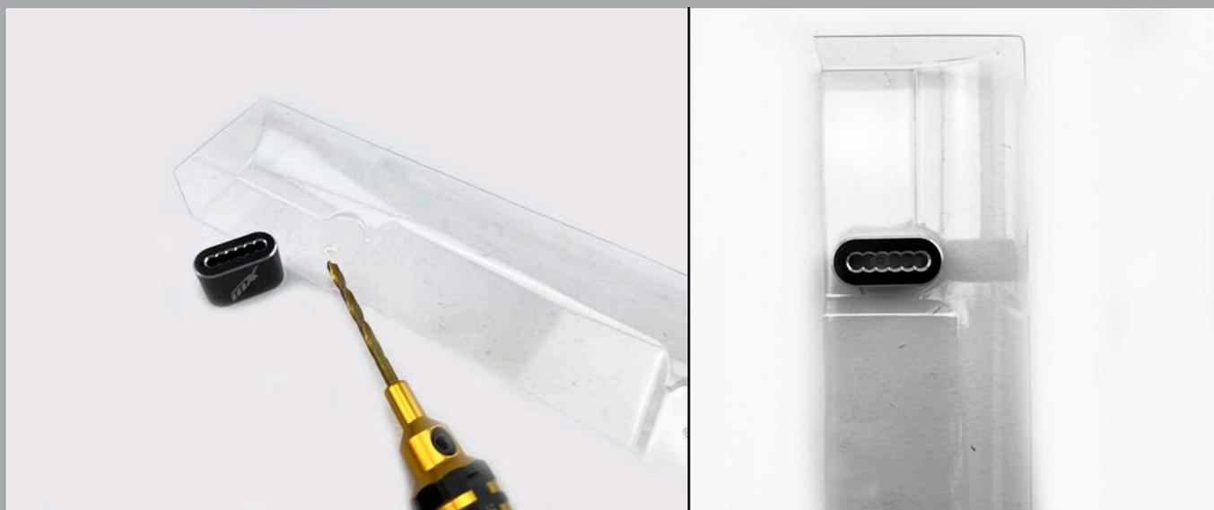
Remind the orientation of the drill jig! Take care to insert the drill bit correctly otherwise it could bind or you even damage the aluminum jig. Start carefully to drill the hole (\*3). Depending on the wing it takes just a few turns to get through (\*2).
