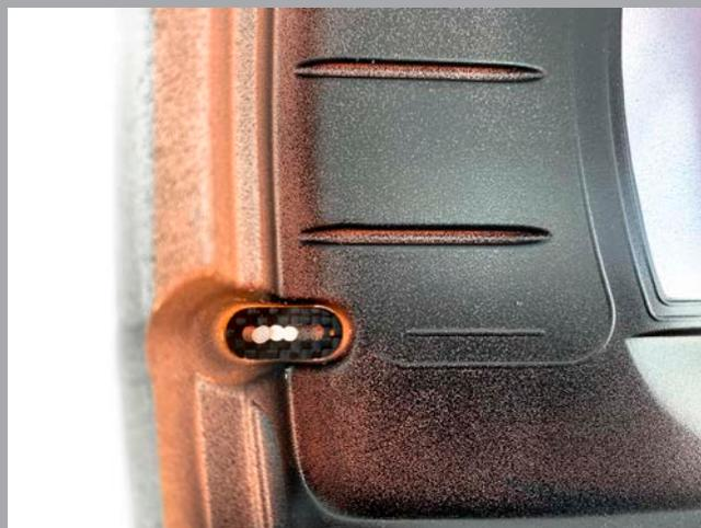
Depending on the Bodyshell thickness (\*2) its possible to drill the holes right after each other. We highly recommend to use the Precision Carbon Wing Mount plates on the in and the outside! The form fit of these plates inside the wing mount will ensure a perfect and stong bolting of the wing.
