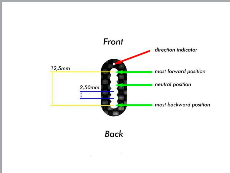
**STEP 4:** Use the 3,0mm Ti-coated drill bit and insert it into your preferred hole position of the aluminum jig. Take care to insert it correctly otherwise it could bind or you even damage the jig. Start carefully to drill the hole (\*3). Depending on the Bodyshell it takes just a few turns to get through (\*2).
