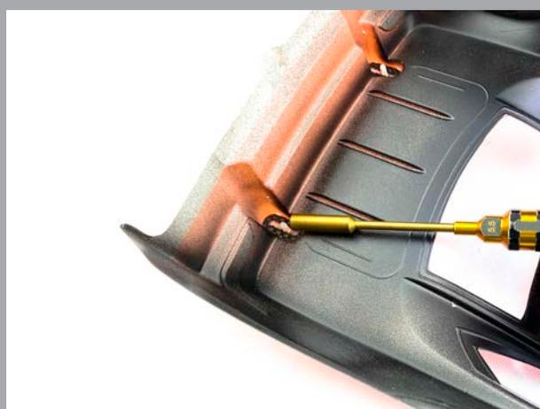
Take care to not overtight the PA nuts (\*4). We recommend to add a second nut (we include enough) on every screw to create a "double nut"-bonding. After STEP 6 you are ready to hit the track! STEP 7 is about additional holes to further adjust the handling.
