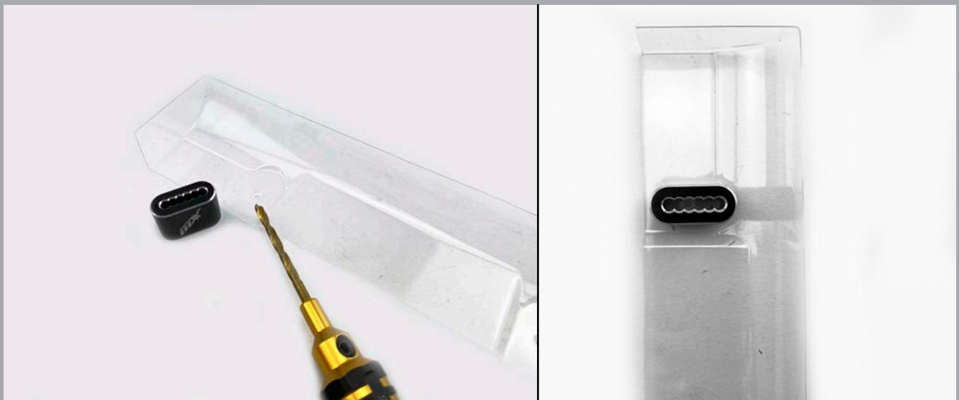
Remind the orientation of the drill jig! Take care to insert the drill bit correctly otherwise it could bind or you even damage the aluminum jig.
