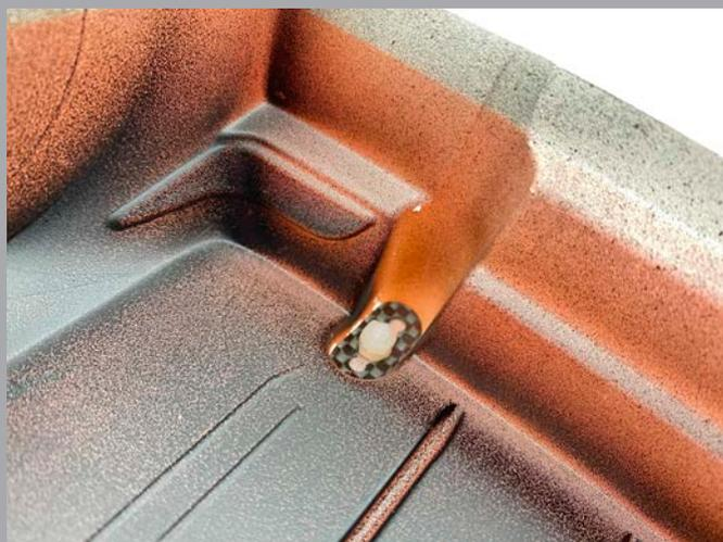
**STEP 7:** If you want to adjust your wing position, either more forward or backward in order to change the handling, you can easily drill additional holes. Remove the rear wing from the Bodyshell and place the aluminum drill jig inside the wing mount. Put the drill bit inside the choosen hole of the jig and drill the additional hole.
