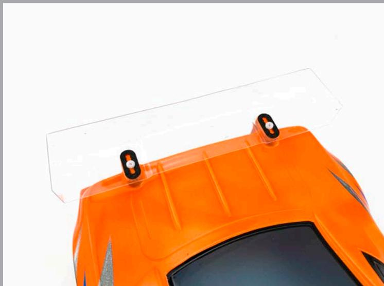
Place another Precision Carbon Wing Mount Plate inside of the Bodyshell. This extend the rigidy of the mount and keep the screw in the correct position, which is even more important if you drilled additional holes. Use a Philips screwdriver and a 5,5mm nut driver to bolt on the wing with the included M3 nuts.
