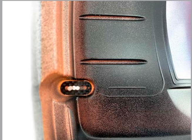
Depending on the Bodyshell thickness (\*2) its possible to drill the holes right after each other. We highly recommend to use the Precision Carbon Wing Mount plates on the in and the outside! The form fit of these plates inside the wing mount will ensure a perfect and strong bolting of the wing.
